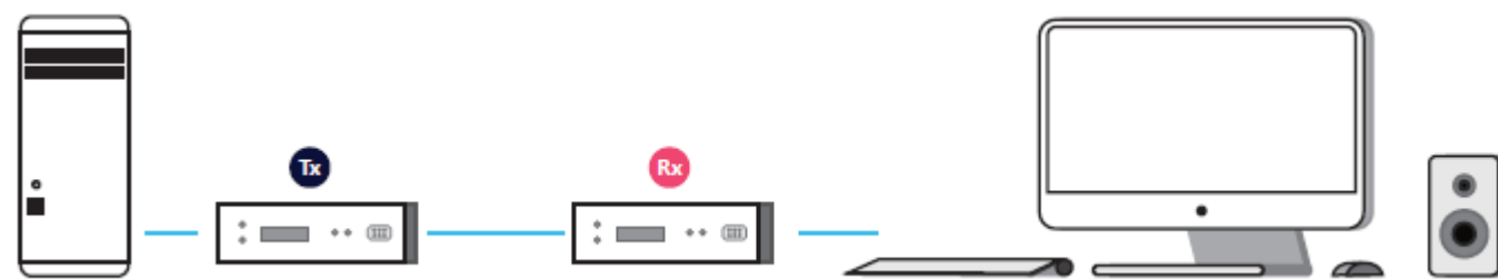
Spot to Spot Mode: Tx – Rx as long distance extension, up to 100m
